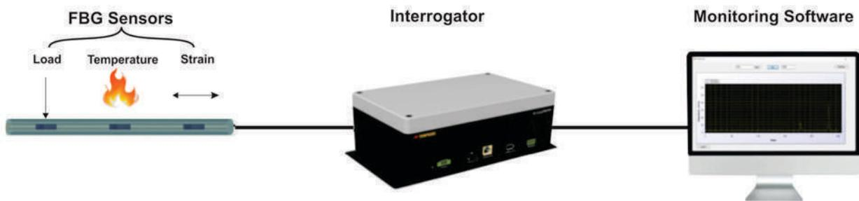
FBG sensor system configuration for Load/Temperature/Strain Sensing
